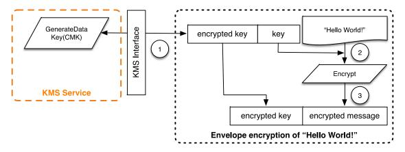
Figure 4: AWS SDK envelope encryption with AWS KMS
