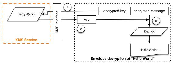
Figure 5: AWS SDK envelope decryption using AWS KMS
